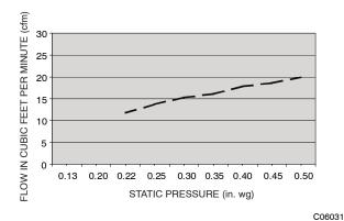
Fig. 78 - Outdoor-Air Damper Leakage
